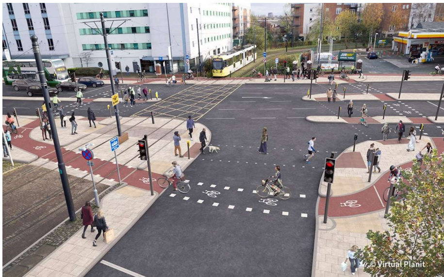
Figure 3-5. CYCLOPS traffic signal junction incorporating a mass transit corridor – Manchester
